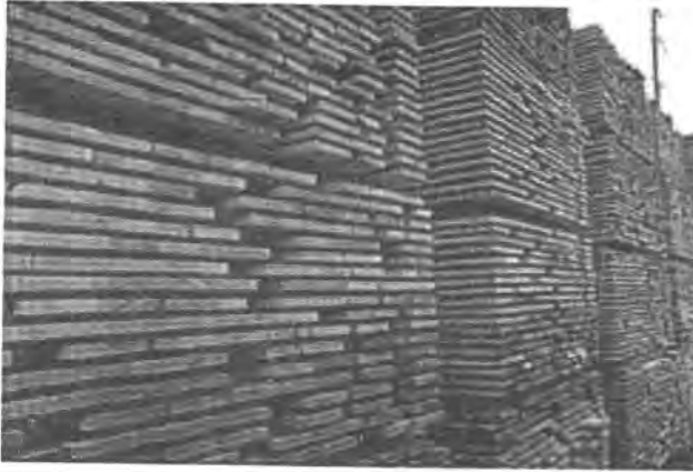
Figure 4. Inspection paths between timber stacks
