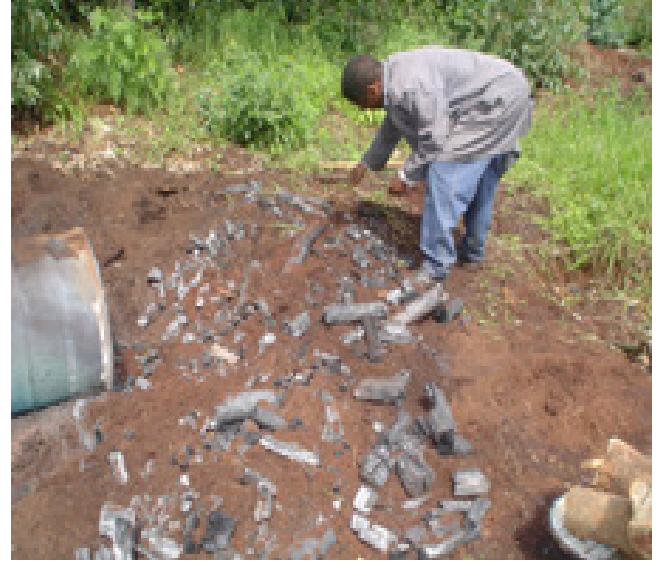
Figure 7. Charcoal removed from drum and covered with soil to cool and prevent burning.
