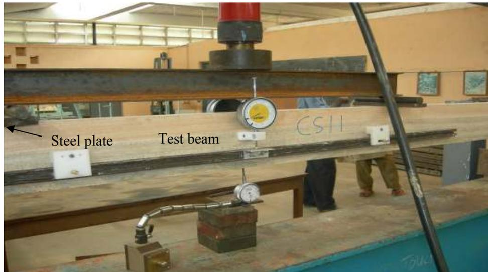
Figure 1b: Typical experimental set-up with instrumentation
