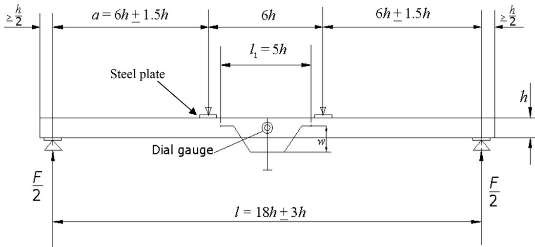
Figure 1a: Schematic test arrangement for measuring local modulus of elasticity in bending
