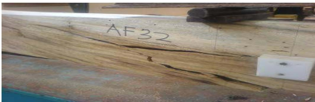
Figure 3: Typical splintering tension failure of an *Albizia ferruginea* beam
