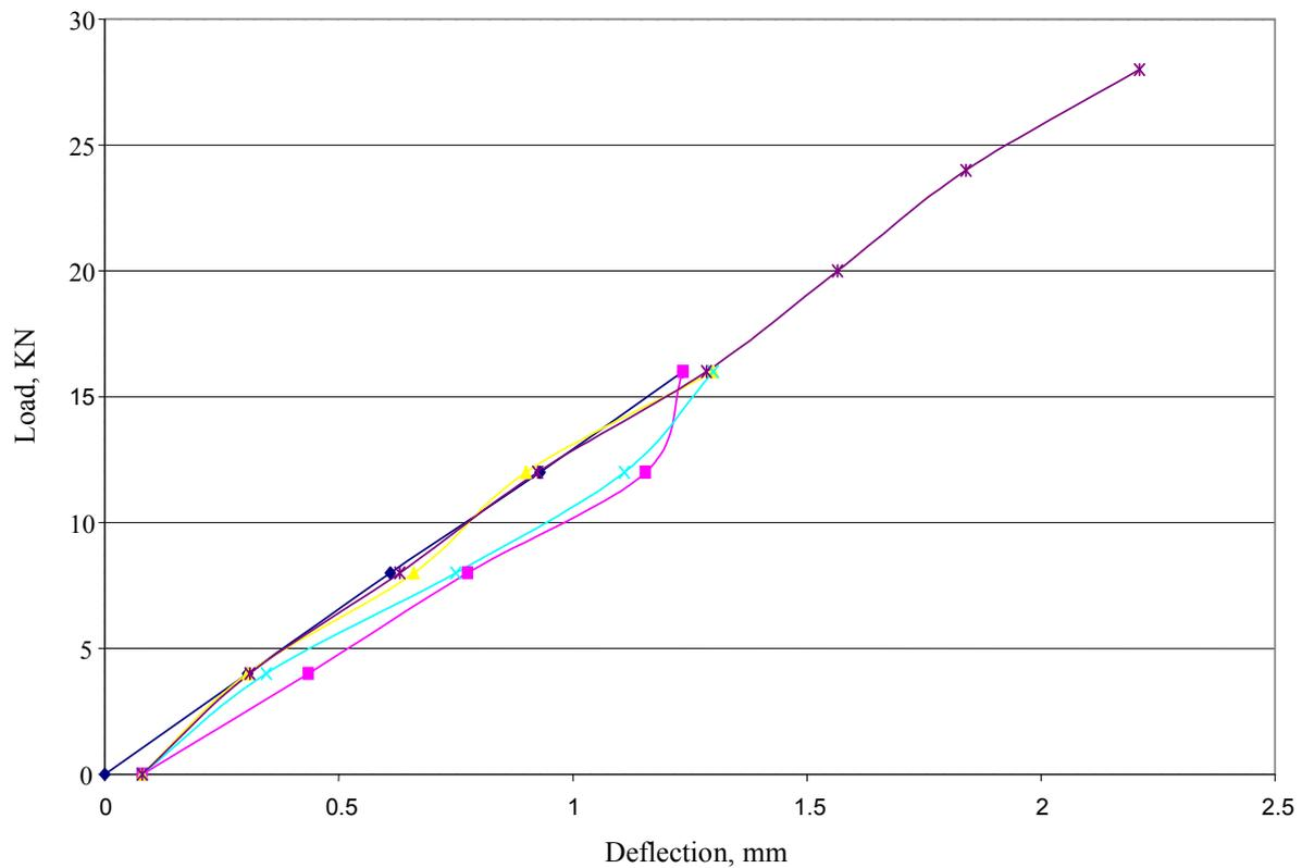
Figure 2: Typical load-deformation curve (SR31local modulus) of the species (L1 = First cycle loading; UI = First cycle unloading; L2 = Second cycle loading; U2 = Second cycle unloading; L3 = Loading to failure)
