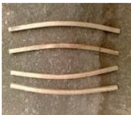
Figure 7a: Danta after steam bending
