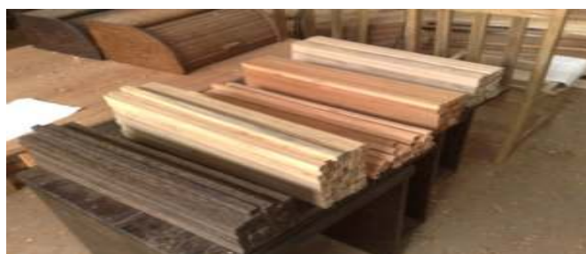
Figure 1: Test specimens of 15mm x 15mm x 500mm dimensions
