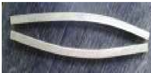
Figure 7b: Rubberwood after steam bending
