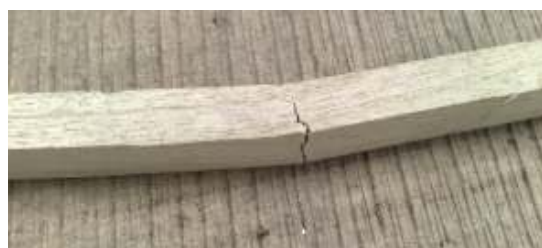
Figure 6b: Brittle tension failure in Rubberwood
