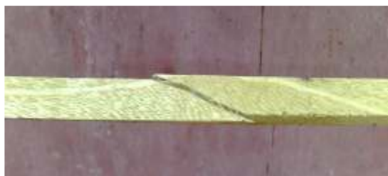
Figure 6a: Cross grained tension failure in Emire
