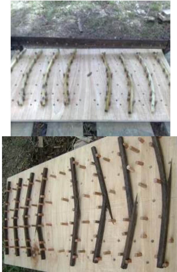
Figure 4: Steam bent specimens on pegged form
