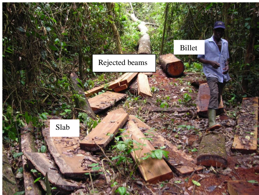
Figure 4: Types of solid wood residue generated during chainsaw milling process. Picture from Nkrabia Forest Reserve showing residue from a sawn mahogany tree
