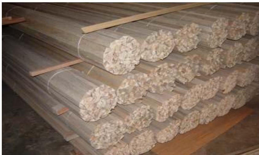
Figure 2: Triangular profiles made from rejected peeler cores
