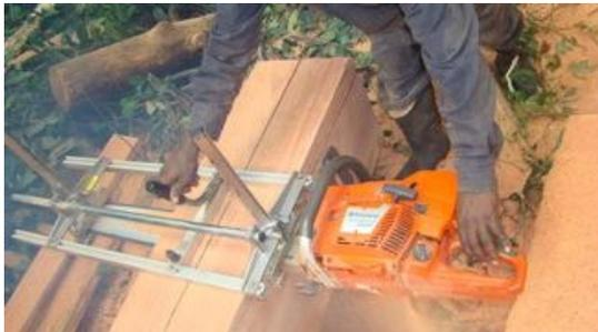
Plate 4: Milling with a frame attachment
