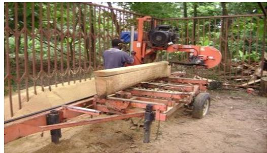
Plate 5: Milling with wood-mizer
