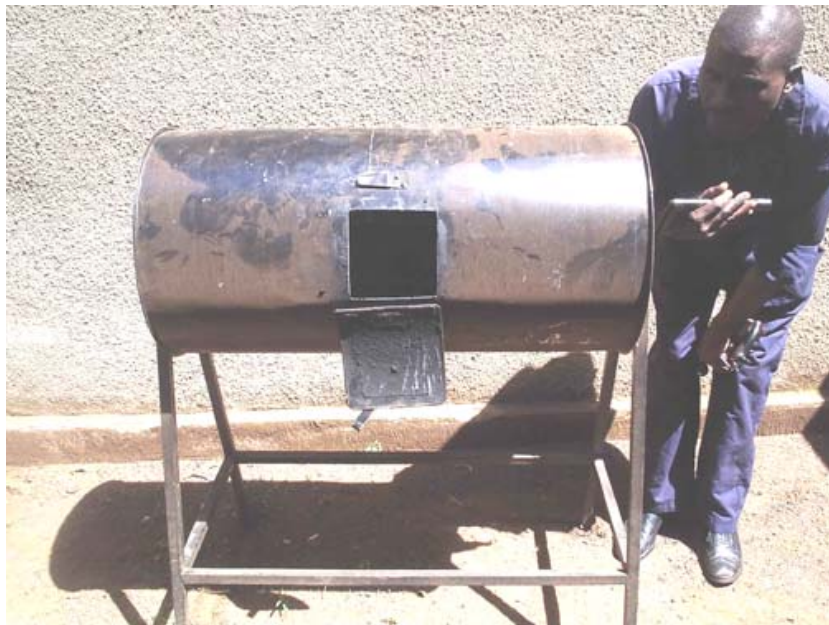
Figure2. Manually operated drum mixer for blending carbonized bagasse and clay
