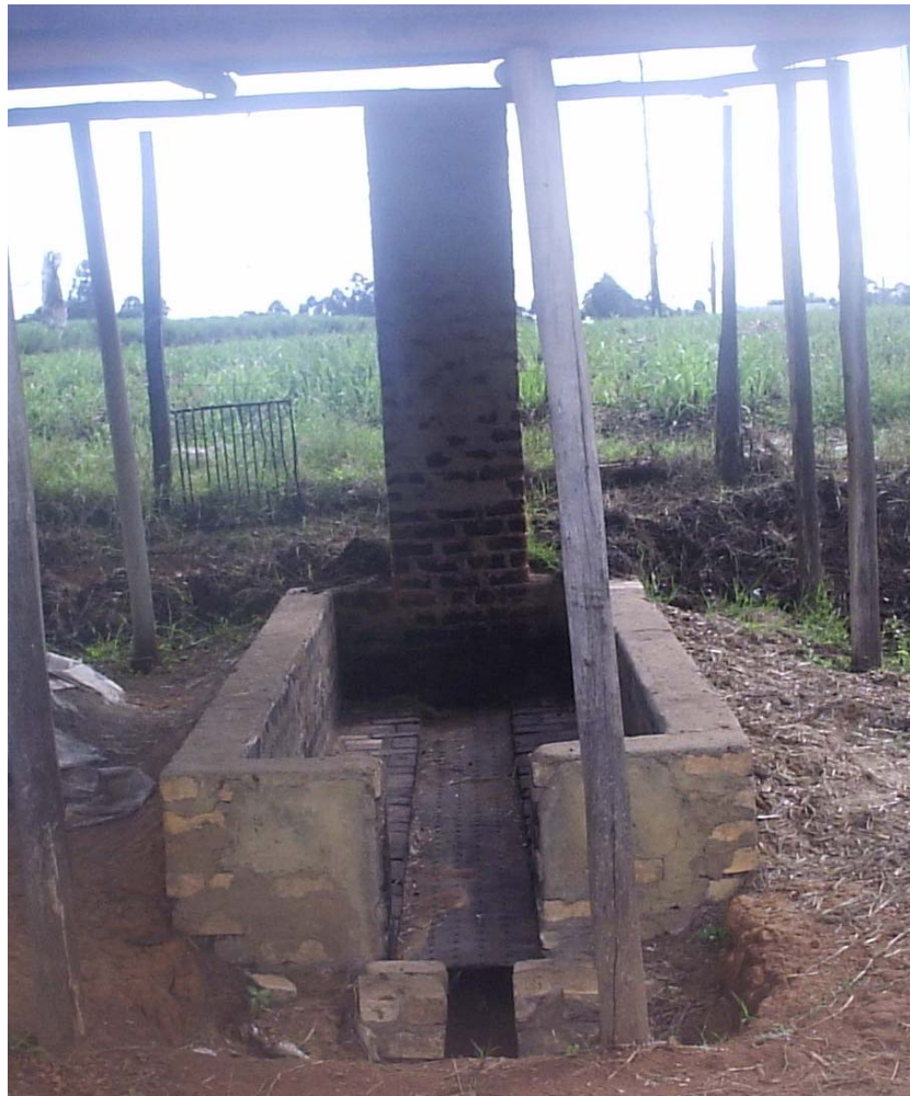
Figure 1. Brick-built kiln used for carbonizing bagasse
