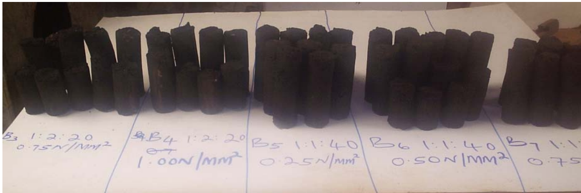
Figure 3. Various briquettes produced using different ratios and pressures
