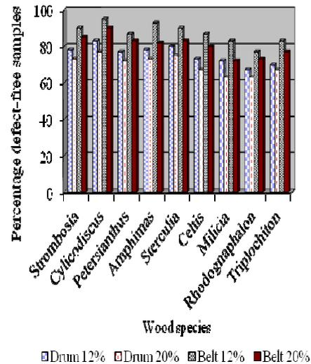
Figure 4: Relative freedom from fuzzing after sanding with grit size 120
