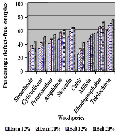
Figure 2: Relative freedom from chipping after sanding with grit size 80
