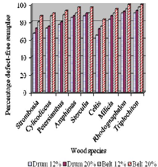
Figure 1: Relative freedom from chipping after sanding with grit size 60
