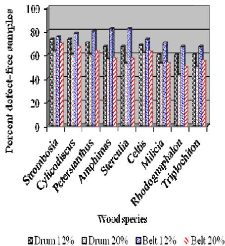
Figure 3: Relative freedom from fuzzing after sanding with grit size 100
